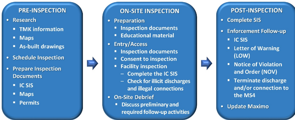
Figure 3-1. Routine Inspection workflow is organized into pre-, on-site, and post-inspection processes.
